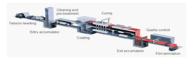
The coil coating process is the most efficient means of coating aluminum with an organic protective coating. It is a continuous, high-volume process that produces a consistent product in comparison to batch post-coating methods. The aluminum substrate gets degreased, chemically pre-treated and coated. Typical paint system requirements are formability, scratch-resistance, appearance, weatherability, printability, etc
